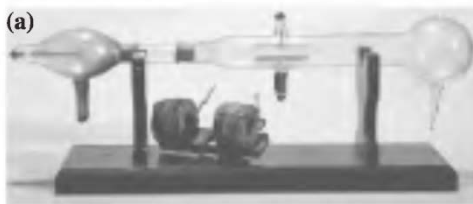
FIGURE 38.7 Thomson's crossed-field experiment to measure the velocity of cathode rays. The photograph shows his original tube and the coils he used to produce the magnetic field.
