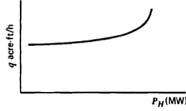
FIG. 7.6 Hydroelectric unit input–output characteristic for constant head.
