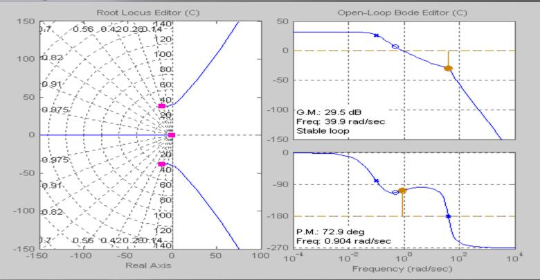
Design with root locus, Bode, and Nichols plots of the open-loop system. Cannot handle continuous models with time delay.
