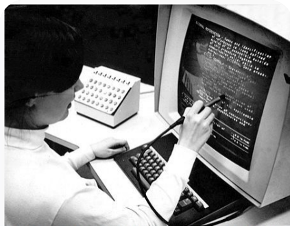
IBM 2250 Model 4 display station, including light pen and programmed function keyboard.
